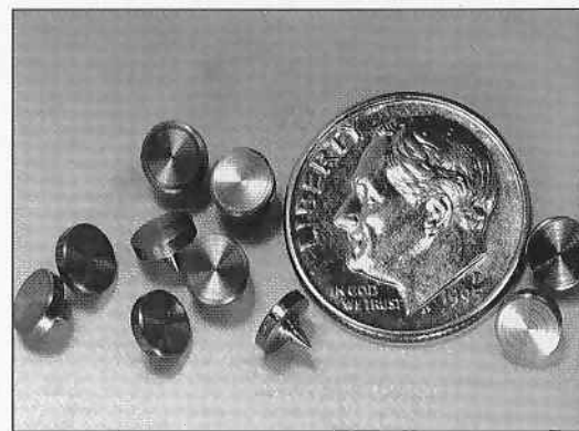
Fig. 1 — Tacks are machined from steel wire and heat treated. Vacuum carburized, hardened, and tempered AISI 11L17 has replaced hardened and tempered 41L40.
